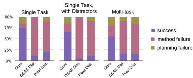
Figure 11: Quantitative performance of visual planning for object rearrangement tasks across different goal specification methods: our meta-learned classifier, DSAE [17], and pixel error. Where possible, we include break down the cause of failures into errors caused by inaccurate prediction or planning and those caused by an inaccurate goal classifier.
