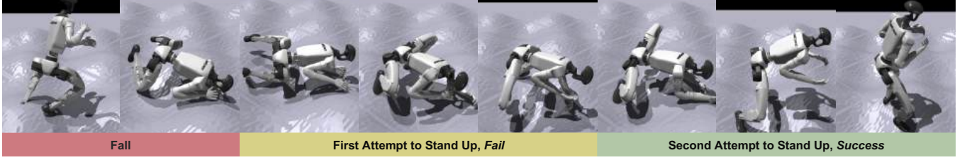
Fig. 10. Re-stand after a failed trial. Instead of terminating upon a failed attempt, the online adapter dynamically re-evaluates the situation and identifies a new intermediate goal to initiate a subsequent re-stand trial.
