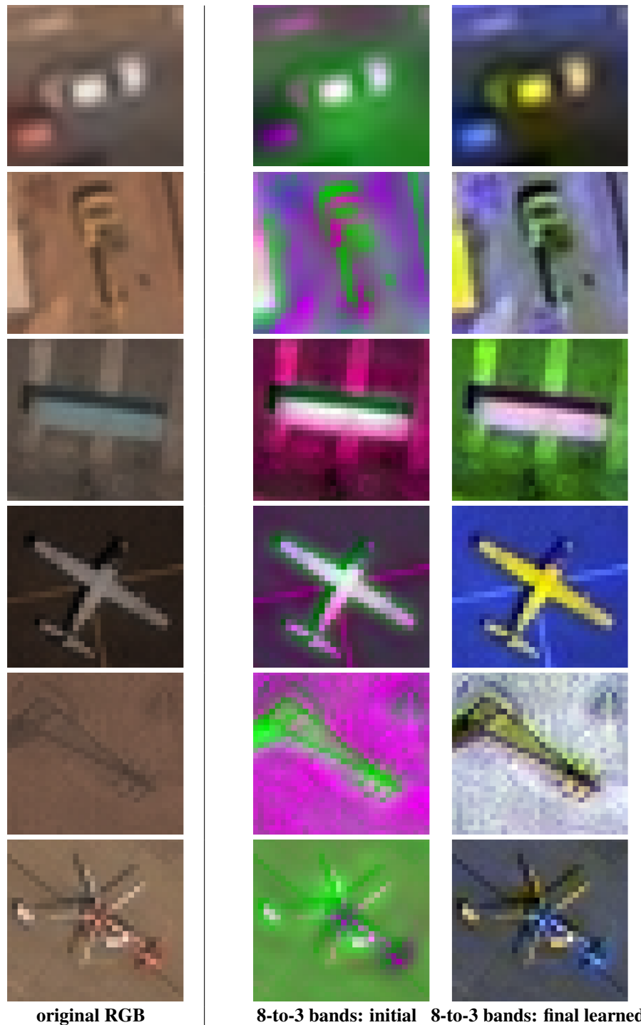
Figure 3: 8-channel input contains useful discriminative information. The 1 \times 1 convolutional filter prepended to the Resnet18 is learning to squeeze the 8-channel input into 3 channels. Column 1: Standard color images of RGB bands. Column 2: Color visualization of the 3-channel output from the 1 \times 1 convolutional filter for randomly initialized Resnet18. Column 3: Color visualization of the 3-channel output from the 1 \times 1 convolutional filter for Imagenet1k pretrained Resnet18. Rows 1-6 contain sample instances from head ( PV, EV ), body ( ShippingContainer ) and tail ( FWAircraft/Fixed Wing Aircraft, Pylon, Helicopter ) classes of the distribution. The final projected 8-band image is able to distinguish between different surfaces and materials where RGB fails.
