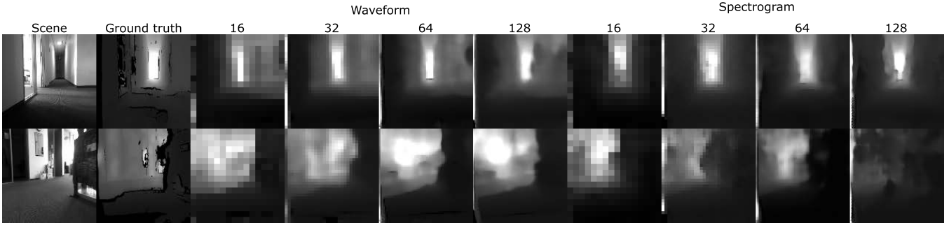
Fig. 6. Sample sound-to-vision predictions by Generator G only without the adversarial discriminator D . Columns 1-2 show the grayscale scene image and the ground-truth depth map. The rest columns show predictions from waveforms and spectrograms at size 16 \times 16 , 32 \times 32 , 64 \times 64 , and 128 \times 128 .
