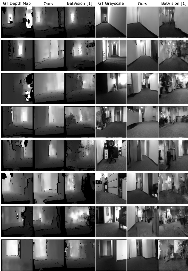
Figure 5. Test sample reconstructions. Columns 1 and 4 show the ground truth depth map and grayscale scene image. The remaining columns show predictions from result from our method and BatVision [1]. Overall, our generations show correct mapping of close and distant areas with less noise and more smooth reconstruction than the BatVision method.
