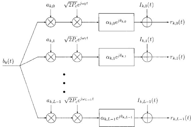
Fig. 2. Equivalent lowpass transmitter and channel for user  $k$ .
