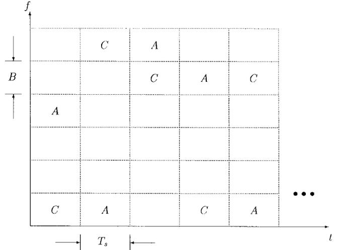
Fig. 7. Allocation of subchannels in an FH/CDMA system to users "A" and "C."
