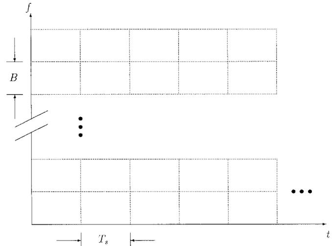
Fig. 1. Time and frequency slot arrangement from the MC approach.
