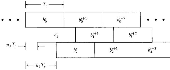
Fig. 5. Asynchronous system bit timings.
