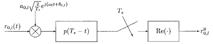
Fig. 6. Correlator demodulation on slot  $l$ .
