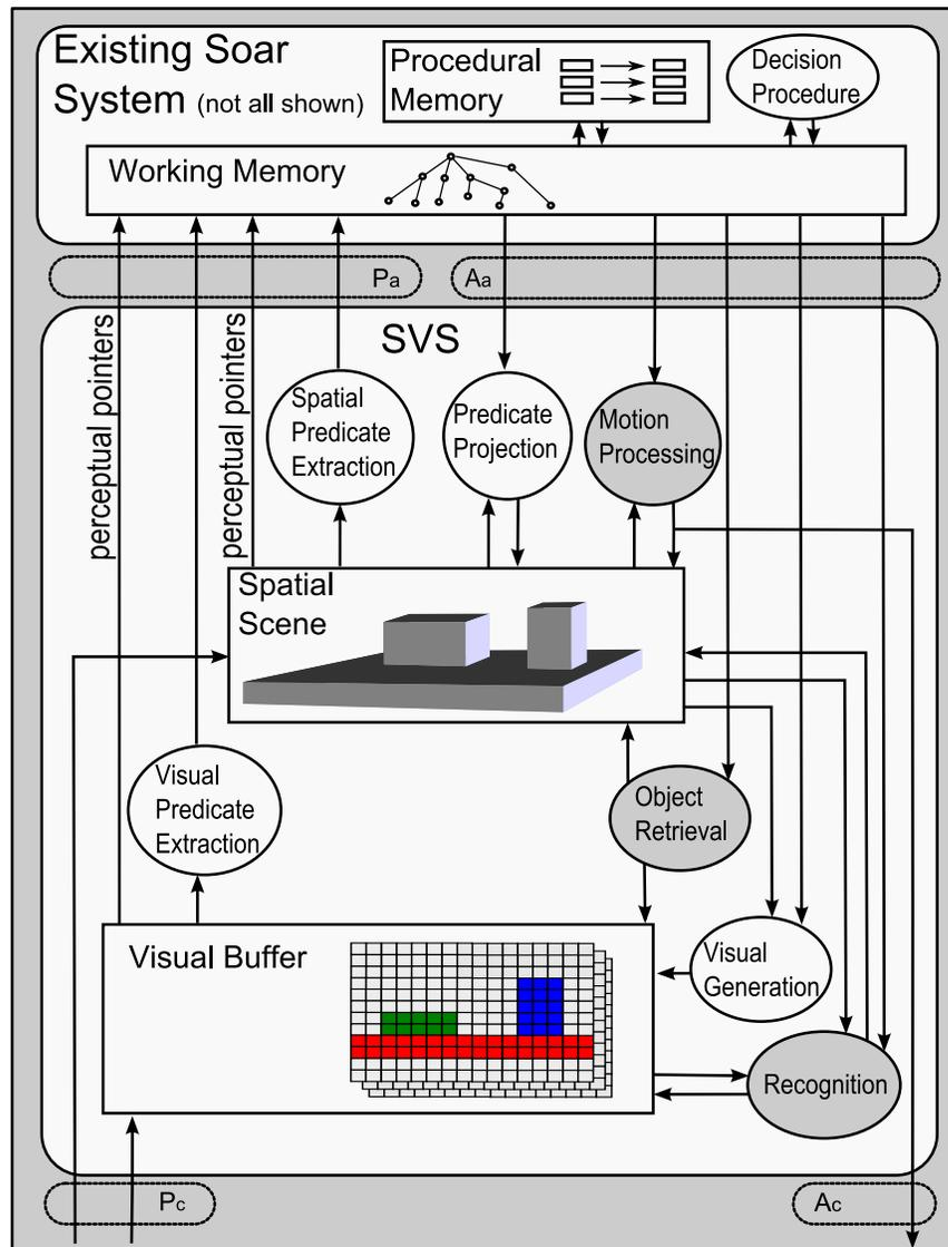
**Figure 8: SVS System design. Boxes are short-term memories, circles are processes. Grey circles involve access to information in long-term memory (knowledge). There are implicit control lines (not shown as arrows) between working memory and all of the processes shown.**
