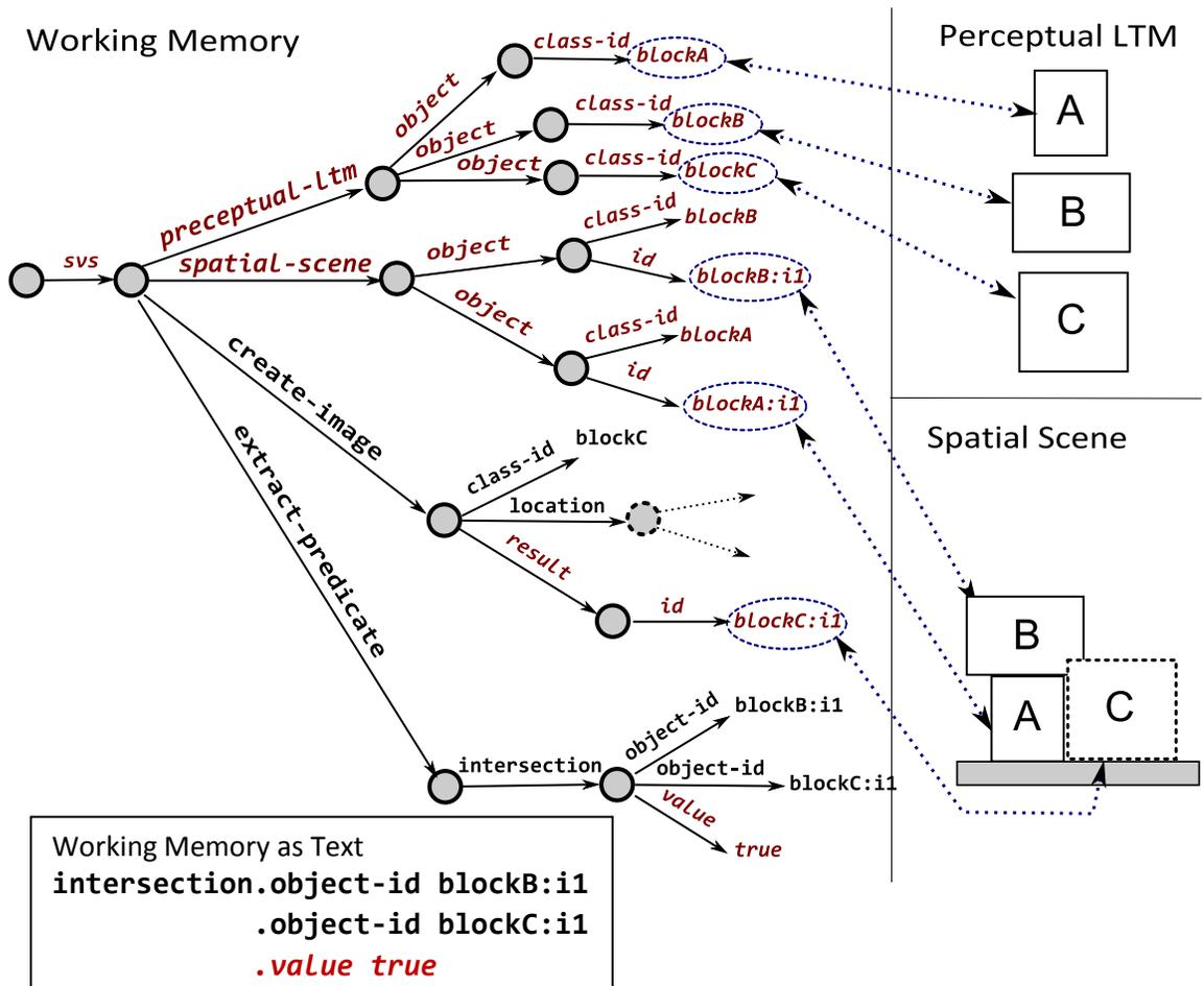
Figure 9: Top, blocks world information in Working Memory, Perceptual LTM, and Spatial Scene. Bottom, equivalent text representation of the extract-predicate structure. Working memory structures in *red italics* are created by SVS.
