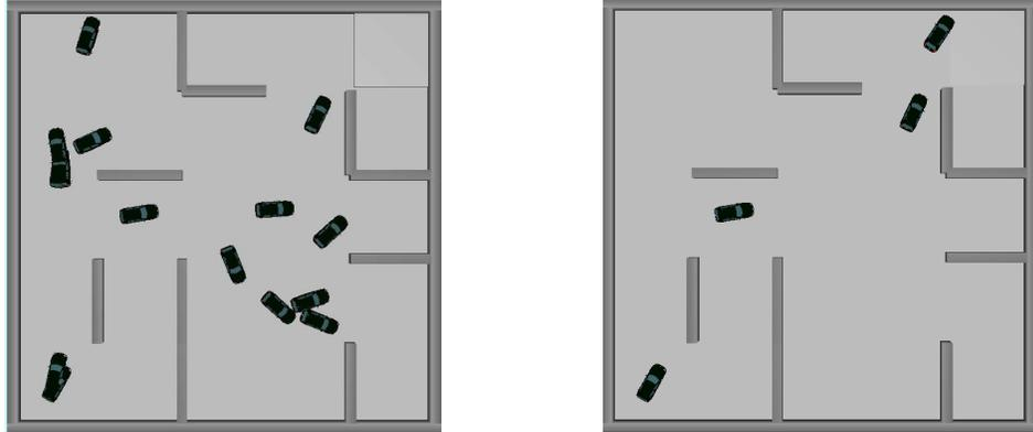
**Figure 25: States of SVS Spatial Scene during RRT planning. The problem is to drive a car from lower-left to upper-right. Left: RRT tree, just before a solution is found. Right: Sequence of car positions that solve the problem.**
