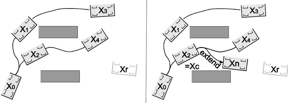
**Figure 24: An example of RRT applied to car motion planning.**
