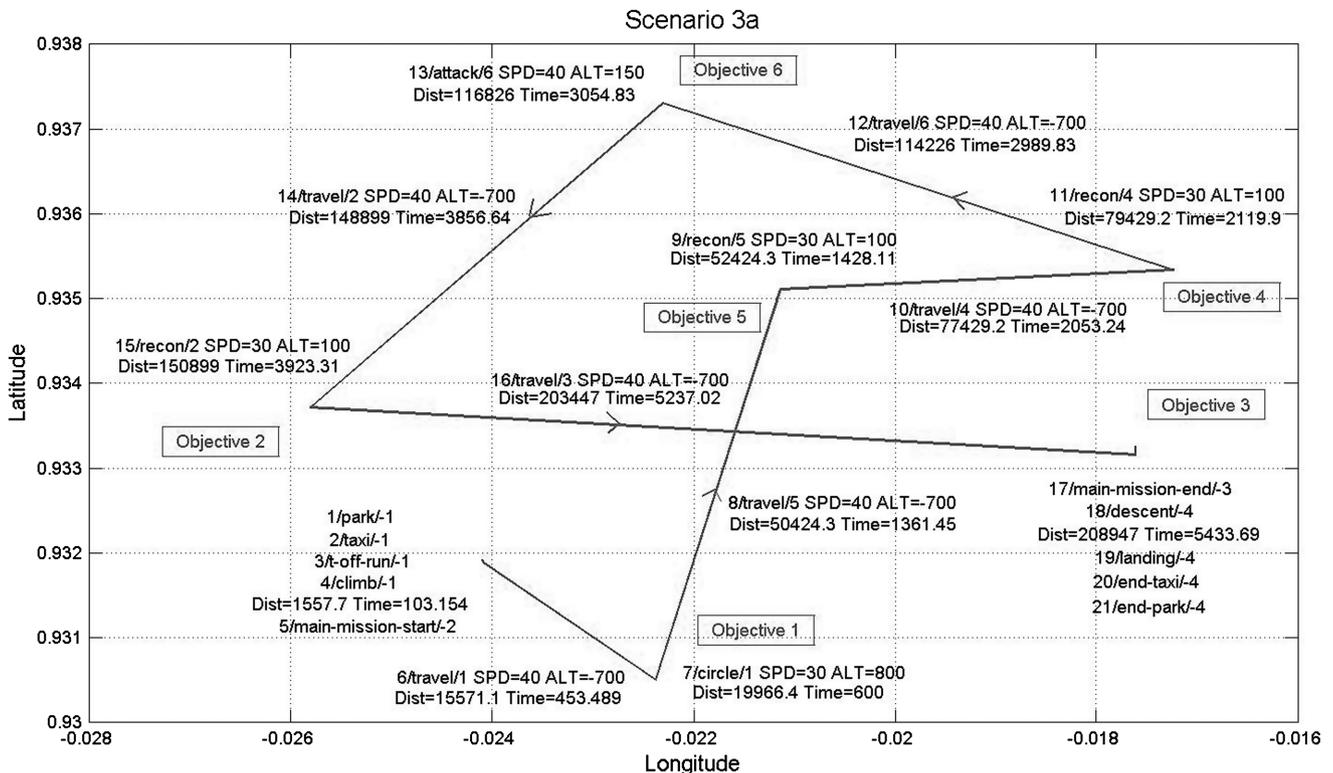
Fig. 7 Plot of initial scenario 3 flight plan (SPD: speed, m/s; ALT: altitude, m).
