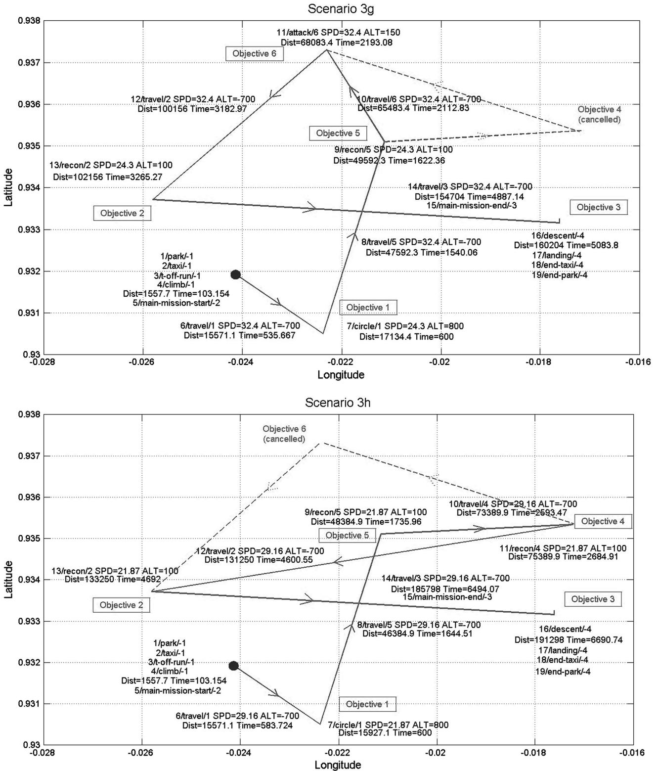
Fig. 12 Plot of scenario variations 3g and 3h flight plan (SPD: speed, m/s; ALT: altitude, m).
