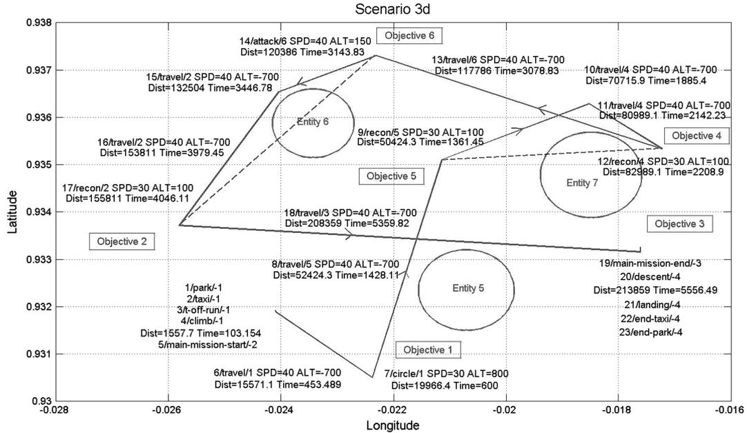
Fig. 10 Plot of scenario variation 3d flight plan (SPD: speed, m/s; ALT: altitude, m).
