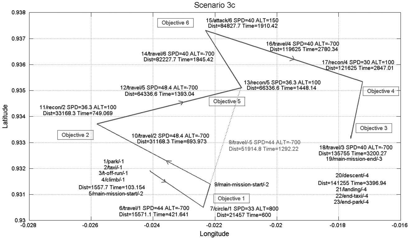
Fig. 8 Plot of initial scenario 3 flight plan (SPD: speed, m/s; ALT: altitude, m).
