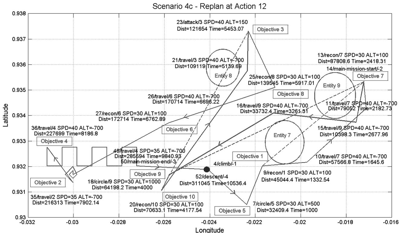
Fig. 15 Plot of scenario 4c flight plan, replanning event at action 12 (SPD: speed, m/s; ALT: altitude, m).
