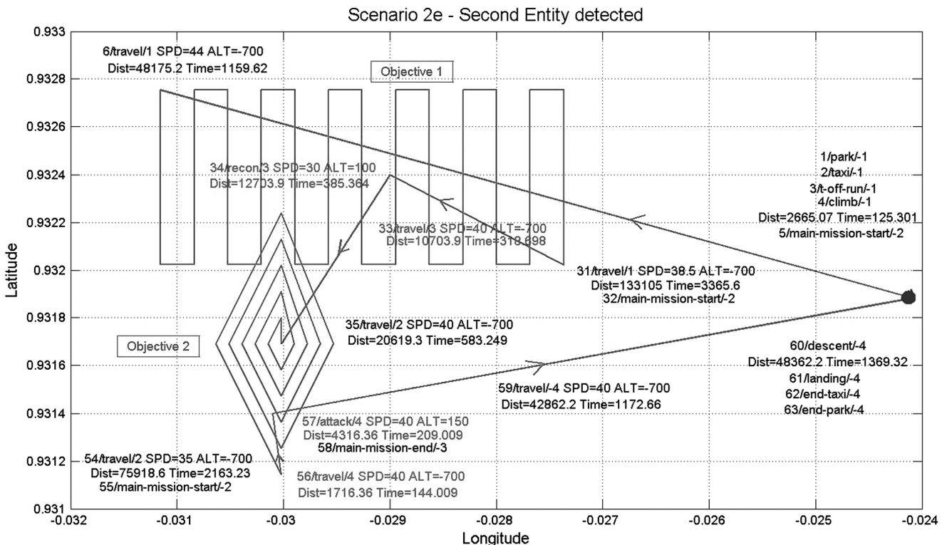
Q4 Fig. 4 Scenario 2e flight plan (SPD: speed, m/s; ALT: altitude, m).
