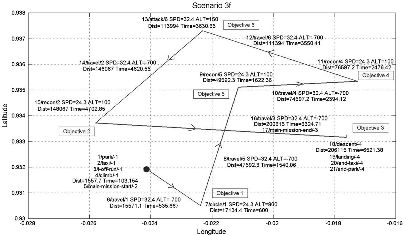
Fig. 11 Plot of scenario variation 3f flight plan (SPD: speed, m/s; ALT: altitude, m).
