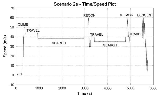
Fig. 6 Speed plot highlighting priority-check algorithm.
