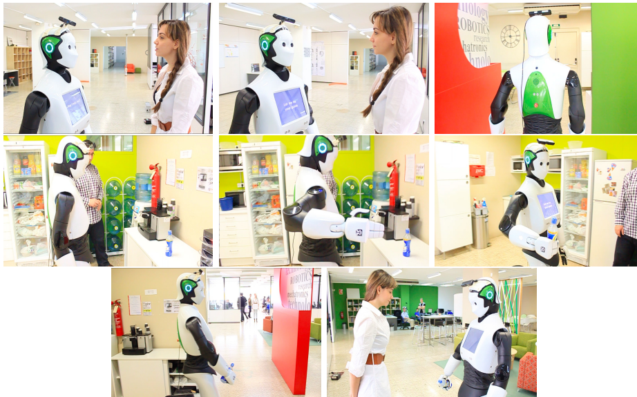
Figure 4. Sequence of actions done by the REEM robot to solve the command “ Bring me a drink ”: Listen to command, request missing information and acknowledge full command, go to kitchen, look for objects, detect energy drink, grasp energy drink, return to master, deliver energy drink.
