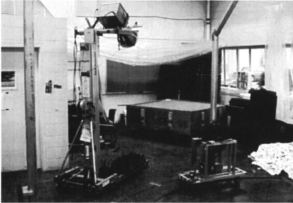
Fig. 2. Photograph of experimental setup. Radar mounted on a mechanical lift overlooking a sandbox filled with the test material. (Additional equipment is part of an unrelated bistatic facility.)
