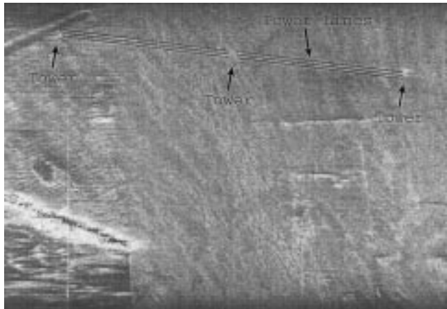
Fig. 10. The SAR image shown in Fig. 9 after detection of power lines.
