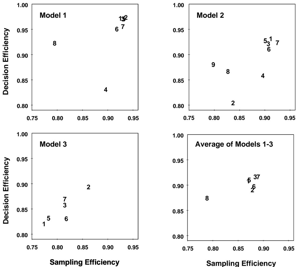
Figure 3: Efficiency Tradeoff Curves: Sampling versus Decision efficiency by Method and Model.  $n = 50$  and  $D = 6$ . Methods that are missing from plots fall below the plot ranges. Methods are: **1.** 2-par MLE; **2.** 1-par Bayes; **3.** 2-par Bayes; **4.** Convex-concave; **5.** Smooth conv-conc; **6.** Monotone; **7.** Smooth monotone; **8.** Up-down; **9.** EA
