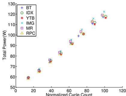
**Figure 1:** Correlation of power with non-halted CPU cycle.
