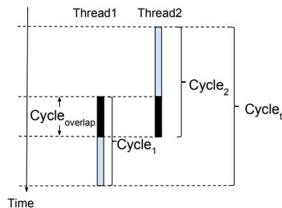
**Figure 4:** Illustration of how we capture the detailed utilization of a physical core using three counters. Thread 1 and 2 are sibling hyperthreads of a physical core, and their non-halted CPU cycles are respectively  $Cycle_1$  and  $Cycle_2$ .  $Cycle_1$  represents non-halted cycles when at least one of the two hyperthreads of a physical core is active.
