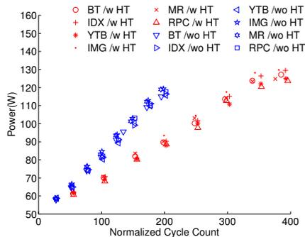
**Figure 2:** Correlation between power and cycle when hyperthreads are enabled.
