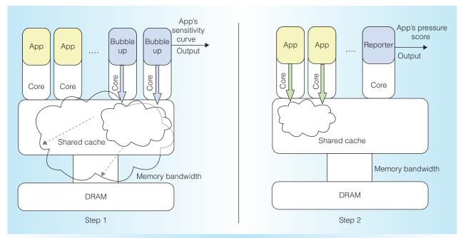
Figure 3. Bubble-Up methodology. In step 1, we characterize the host application task's sensitivity to pressure in the memory subsystem using a bubble. In step 2, we characterize the host application's contentiousness in terms of the pressure it causes on a reporter.
