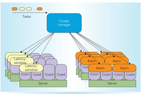
Figure 2. Task placement in a cluster. The cluster manager doesn't colocate latencysensitive applications with others to protect their quality of service (QoS) from performance interference, causing low machine utilization.
