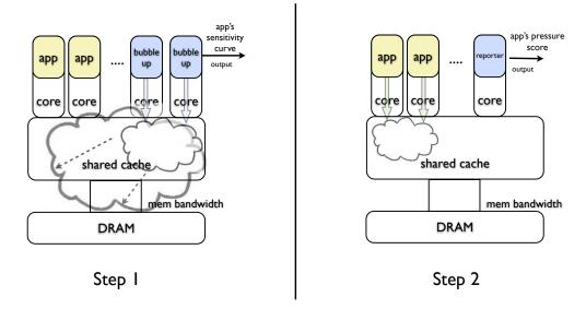
Figure 4: Bubble-Up Methodology. In Step 1, we characterize the sensitivity of the host application task to pressure in the memory subsystem using a bubble. In Step 2, we characterize the contentiousness of the host application in terms of the amount of pressure it causes on a reporter.
