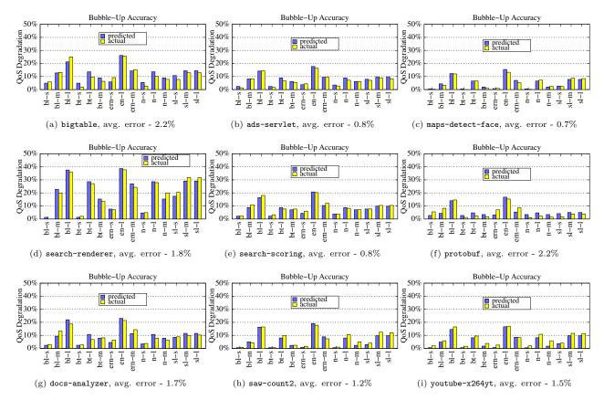
Figure 10: The Accuracy of Bubble-Up in Predicting QoS Impact for 9 Highly Sensitive Google Workloads.
