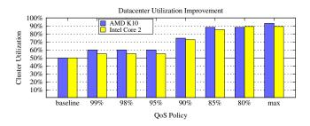
Figure 16: Improved utilization in a clusters composed of AMD K10 Opteron servers and Intel Core 2 Xeon servers.
