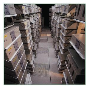
Figure 4. I 00-node 200-CPU cluster. Key design points include extreme symmetry, internal disks, no people, no monitors, and no visible cables.
