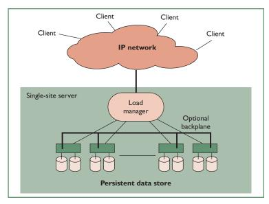
Figure 1.The basic model for giant-scale services. Clients connect via the Internet and then go through a load manager that hides down nodes and balances traffic.
