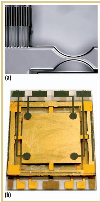
Figure 4. Two electrostatic generators fabricated in microelectromechanical systems: (a) a portion of a constant-gap variable capacitor fabricated at MIT for a 1 cm<sup>2</sup> device and (b) a 2 cm<sup>2</sup> compressible-plate capacitor fabricated at Imperial College. (figure 4a photo courtesy of Anantha Chandrakasan and Jeff Lang, MIT Microsystems Technology Lab; figure 4b photo courtesy of Peng Miao)
