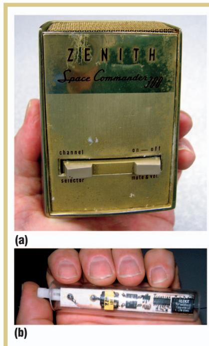
**Figure 5.** Self-powered wireless pushbutton remote controls: (a) A 1956 Zenith *Space Commander*, a passive ultrasound transmitter, and (b) the MIT Media Lab's self-powered wireless switch, which sends a digitally coded radio frequency stream.
