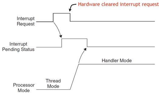
The normal case. Once Interrupt request is seen, processor puts it in "pending" state even if hardware drops the request. IPS is cleared by the hardware once we jump to the ISR.
