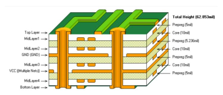
Vias (plated holes) allow signals to move between the layers
