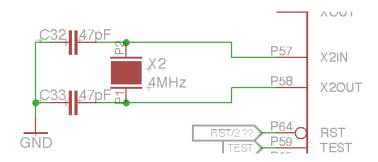
$$C_L = \frac{C_{X1} * C_{X2}}{C_{X1} + C_{X2}} + C_{stray}$$
