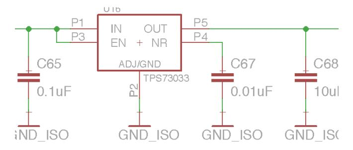
Low ESR requirement means use at least one ceramic cap, close to the IC
