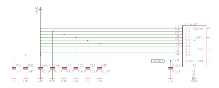
Microprocessor App Note will describe decoupling requirements, location is key!
