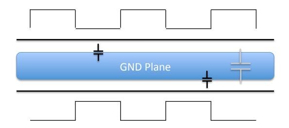
Either way, solve it with a ground plane (copper poured in-between and connected to GND):
