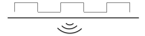
A high speed digital signal in a wire will act as an antenna
