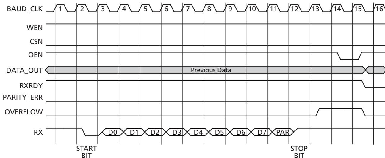
Figure 4-4 · Overflow Error
