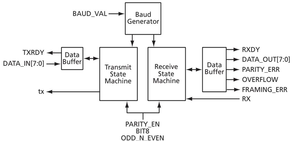
Figure 1-1 · Block Diagram of CoreUART Normal Functionality
