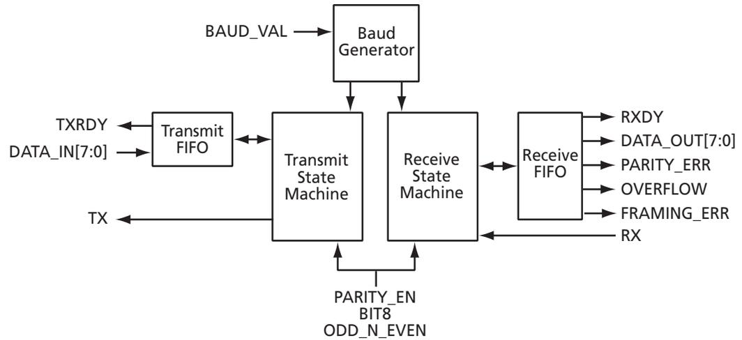
Figure 1-2 · Block Diagram of CoreUART with FIFO Functionality
