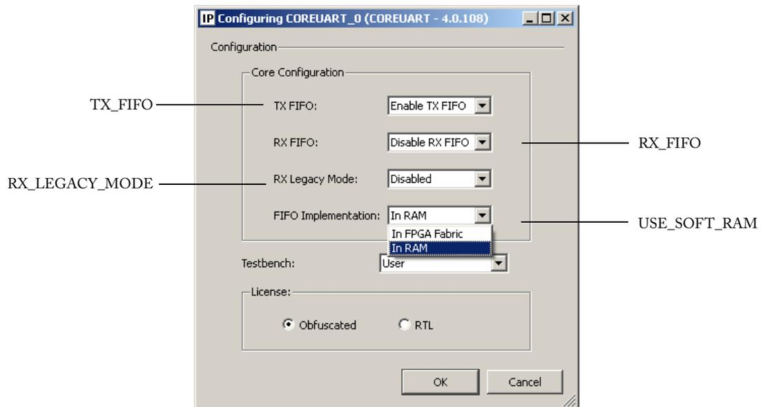
Figure 2-1 · CoreUART Configuration Window
