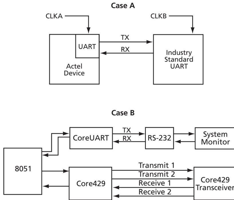
Figure 1 · System Block Diagram Depicting CoreUART Usage
