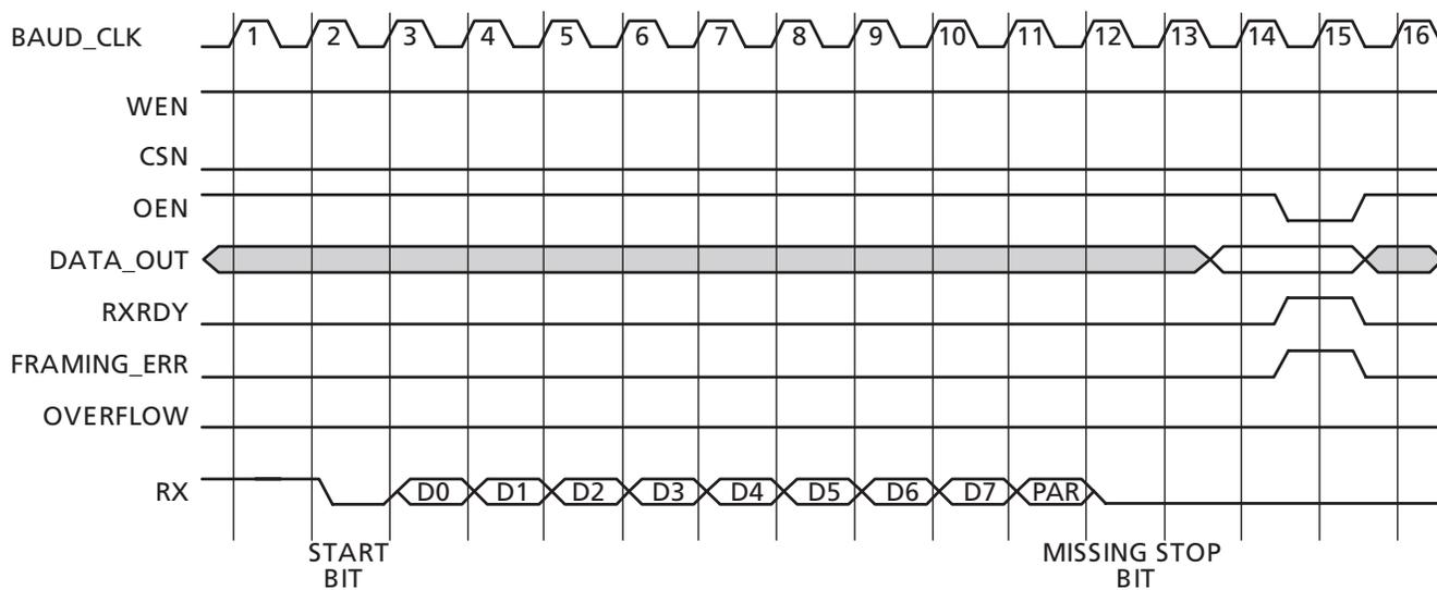
Figure 4-5 · Framing Error
