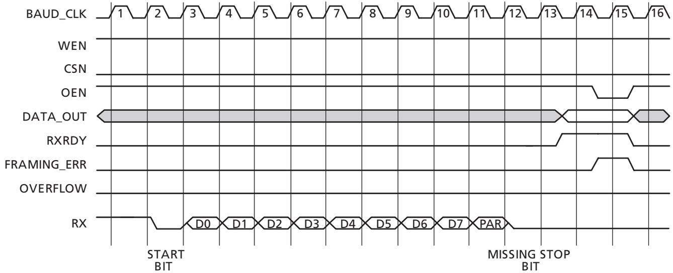
Figure 4-6 · Framing Error in Legacy Mode
