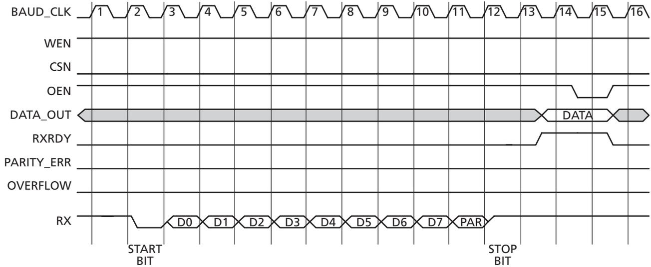
Figure 4-2 · Serial Receive
