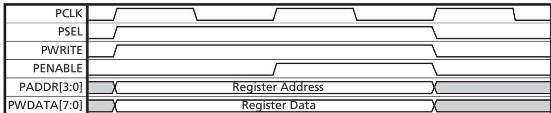
Figure 3-2 · APB Data Write Cycle
