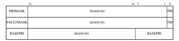
Implementations can support an IMPLEMENTATION DEFINED number of priorities in powers of 2. Where fewer than 256 priorities are implemented, the low-order bits of the BASEPRI field corresponding to the unimplemented priority bits are RAZ/WI.
