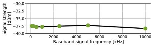
Figure 14: *Impact of baseband signal frequency.* Varying of the baseband signal frequency does not significantly affect the mixed signal strength.
