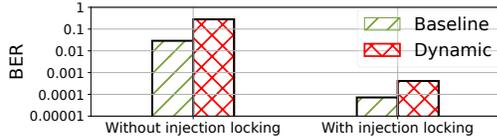
Figure 19: Link reliability of JUDO transmitter in the dynamic environment. When we operate in the without emitter device mode, we observe a significant increase in the number of lost packets and BER. Injection locking the TDO enables us to improve its stability, and consequently, the reliability. NLoS setup and blocked by a building. We position the receiver at a distance of 15 m to 105 m from the JUDO transmitter in LoS.
