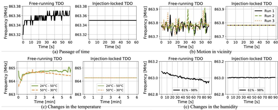
Figure 9: Stabilizing tunnel diode oscillators through injection locking phenomenon. Due to the trade-offs made to lower the power consumption of the TDO, it is unstable and prone to environmental changes (humidity, temperature). By injecting an external carrier signal into the TDO, the stability of the TDO is enhanced.
