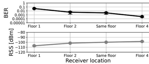
Figure 17: *Link quality (Indoors, bistatic)*. Even with a weak carrier signal, JUDO transmitters offer long-range capabilities. When reflecting a carrier signal, the JUDO transmitter is able to transmit to multiple floors.
