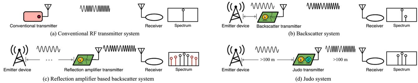
**Figure 2: Comparing JUDO transmitter against transmitters commonly employed on WES.** JUDO allows low-power transmissions while being spectral efficient. Unlike backscatter systems, JUDO allows the emitter device and receiver to be placed at considerable distances from the JUDO transmitter even at high bitrate (100 kbps). In contrast to reflection amplifiers based backscatter transmitters, it does not generate unwanted harmonics (harmonics are shown in red on the spectrum plot).
