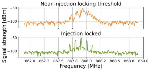
Figure 10: Injection-locking stability. The instability of the TDO (distorted signal) is observed at the threshold of the injection locking state.
