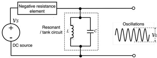
Figure 4: Oscillator designed using a negative resistance element. When a negative resistance element is coupled to a resonant circuit, sustained oscillations result. The frequency of the oscillations is governed by the characteristics of the resonant circuit and the negative resistance element.
