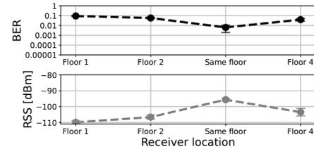
Figure 21: Link quality without emitter device (Indoors, bistatic). Even without an external carrier signal, we can transmit to several floors of a building. It was necessary to configure the receiver frequency regularly to counter drift.
