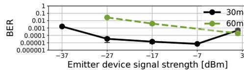
Figure 15: *Link reliability in the monostatic configuration.* We evaluate the link metrics with the JUDO transmitter configured to low-bitrate (3 kbps). We vary the strength of the carrier signal. Link quality, as expected, worsens with the distance of JUDO transmitter from the emitter device.
