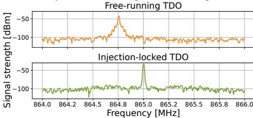
**Figure 8: Injection locking a tunnel diode oscillator.** A free-running TDO produces a noisy signal with a broad peak of the carrier signal. The stability is improved by injection locking the TDO to an external carrier signal. Therefore, we observe a sharper peak of the carrier signal generated by the TDO.
