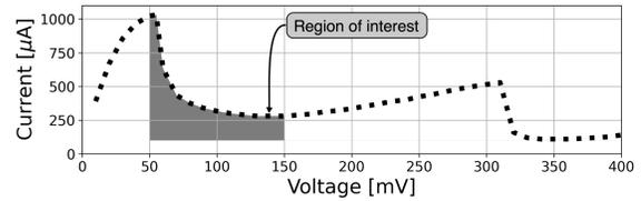
Figure 5: Characteristics of a tunnel diode GE 1N 3712 ( $IV$ ). Tunnel diodes show region of negative resistance, which occurs at low bias voltages and currents. The shaded area of the  $IV$  curve represents the region that leads to oscillations in the tunnel diode oscillator.
