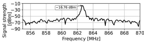
**Figure 7: Tunnel diode oscillator spectrum.** The tunnel diode oscillator generates a carrier signal in the 868 MHz frequency band. The strength of the carrier signal (on average) is  $-19$  dBm. In this plot, since no injecting carrier signal is present, TDO is noisy and the carrier signal has a broad peak.
