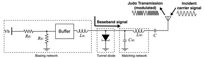
Figure 6: JUDO transmitter schematic. The TDO is a critical component of the transmitter. Locally, the TDO generates a high frequency carrier signal within the 868 MHz frequency band. An external carrier signal provides stability to the TDO. Finally, the self-oscillating mixer property enables mixing of the analog baseband signal with the locally generated carrier signal under 100  $\mu$ Ws.
