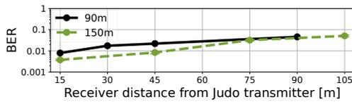
Figure 18: Link quality (Outdoors, bistatic). The distance between the JUDO transmitter and emitter device, and the JUDO transmitter and receiver, can be over 100 m. As compared to backscatter systems, the transmission range is less dependent on the carrier signal strength.
