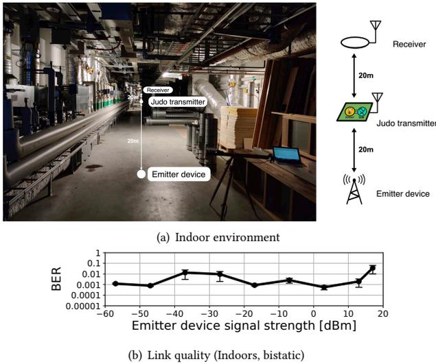
Figure 16: *Link quality (Indoors, bistatic)*. Even in a multi-path rich and challenging radio environment, JUDO transmitters maintain high link quality. However, the link metrics deteriorate at higher carrier signal strengths due to significant self-interference from carrier signal to JUDO transmissions.
