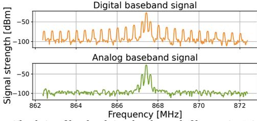
Figure 11: The choice of baseband signal and spread of harmonics. It is possible to eliminate unwanted harmonics generated during the mixing process using an analog baseband signal instead of a digital baseband signal.
