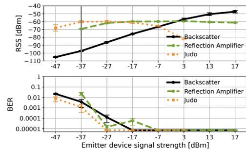
Figure 13: Signal strength and link reliability comparison between transmitters. This is done by varying the carrier strength of emitter device. JUDO significantly outperforms the backscatter transmission when the carrier is weak.
