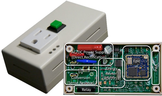
Figure 3. Wireless AC plug-load meter.
