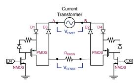
Fig. 6: Current transformer multiplexing circuit responsible for switching the CT between harvesting and measurement operation. When EN is high, the NFETs connect the inputs of the CT across  $R_{BRDN}$  through diodes D1-D4 and enable current sampling. When EN is low, the PFETs stay off and harvesting is enabled. Multiplexing the current transformer is essential for saving size and cost by requiring only a single CT.
