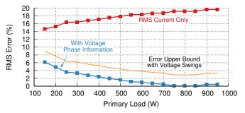
Fig. 14: Error with and without voltage phase information. For a range of loads with power factor of 0.85, the RMS error of Triumvi's power measurement using only RMS current and using sampled current plus voltage phase information is shown. Without any voltage information the error averages 18.5% RMS, and with phase information the average error is 2.5% RMS.
