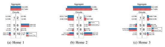
Fig. 17: Short-term deployments in three homes. The energy consumed by each circuit and the aggregate was measured over the course of approximately 2.5 days. Across all of the circuits, our system shows an error of 3.7%. This level of accuracy is sufficient for energy audits, and is capable of providing insight on where additional metering may be warranted.
