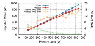
Fig. 13: Comparison with the Pressac CT current meter [10] over a range of 0.85 power factor loads. Power for the Pressac device is calculated by multiplying the reported RMS current values by RMS voltage. Above 250 W, Triumvi's error is significantly lower than the Pressac device. With non-unity power factors, calculating true power is critical for obtaining accurate power measurements.
