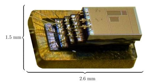
Figure 5.5: **Temperature sensing system.** A system designed as part of the Michigan Micro Mote project consisting of a  $2\,\mu\text{AH}$  battery, a  $900\,\text{MHz}$  near-field radio, an ARM Cortex M0 processor, and an ultra-low power temperature sensor, interconnected using MBus.
