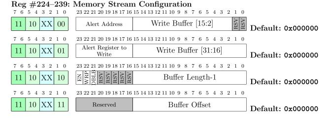
In MPQ each node has up to four independent, identical memory streaming channels. Each channel has two configuration registers. The two registers work together to configure each channel.
