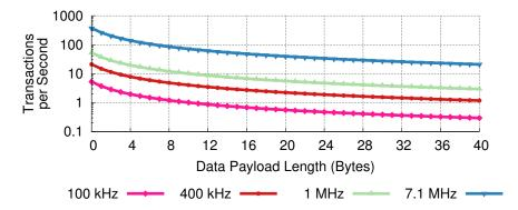
Figure 5.7: **Saturating transaction rate.** As a shared medium, MBus can only support a finite number of transactions across all member nodes. The peak transaction rate depends on the transaction size and bus clock speed.
