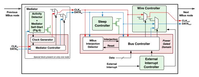
Figure 3.2: Conceptual frontend. A simplified view of the MBus frontend. The default configuration "shoots-through" DATA and CLK signals. Note that there are no local clocks or buffers (beyond generic I/O buffers and drivers) in the MBus ring.
