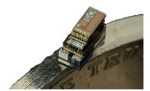
Figure 1.1: Examples of Smart Dust systems. Three millimeter-scale sensing systems composed using the modularity and system design principles outlined in this dissertation.
