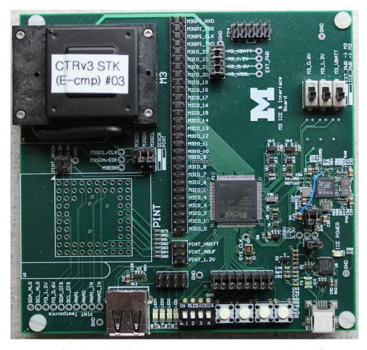
Figure 6.3: **The ICE board.** A custom hardware board that allows flexible hardware access. It supports both traditional in-circuit emulation tasks as well as more general purpose debugging and programming of arbitrary hardware in the greater M3 Smart Dust ecosystem.
