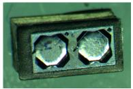
Figure 6.4: A pressure sensor encapsulated in bio-compatible epoxy. Deployment considerations for Smart Dust systems limit the capacity to physically interface with devices.
