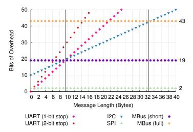
Figure 5.3: **Bus overhead.** MBus message overhead is independent of message length. MBus short-addressed messages become more efficient than 2-mark UART after 7 bytes and more efficient than I<sup>2</sup>C and 1-mark UART after 9 bytes. MBus scales efficiently to messages such as 28.8 kB images (Section 5.3) or longer.
