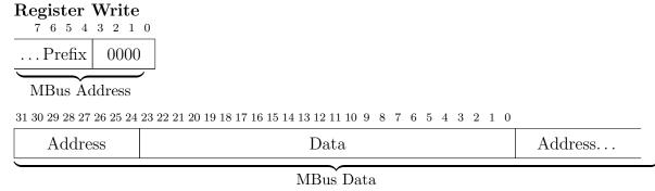
Bits 0-23 of the MBus data field are written to the register addressed by bits 24-31. The write occurs immediately, as soon as the layer controller receives the message. Multiple registers may be written in a single MBus transaction by sending multiple data packets. Each 32 bit chunk of data is treated as if it were an independent transaction.
