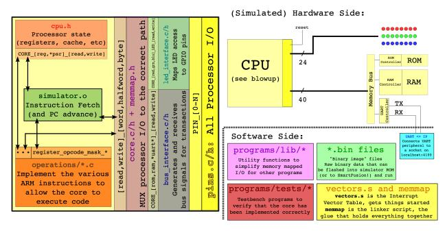
Figure 6.2: **High-level design of M-ulator.** The architecture of M-ulator mirrors that of real hardware. This allows for runtime modularity, where individual components can be implemented either via software emulation or as pass-throughs to real hardware. It further serves a pedagogical goal, as it allows laboratory and project work to explore and implement normally tightly-integrated components in isolation.
