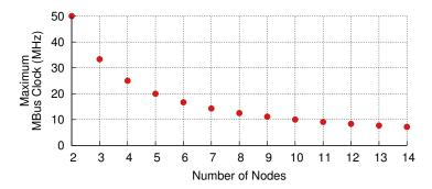
Figure 5.2: **Maximum frequency.** MBus peak clock frequency is inversely proportional to the number of nodes. MBus limits node-to-node propagation delay to 10 ns. For the maximum of 14 short-addressed nodes, MBus could support a 7.1 MHz bus clock.
