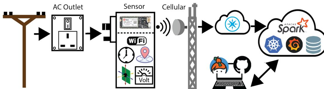
Figure 4.2: **PowerWatch System Architecture.** PowerWatch measures the grid by plugging in at outlets in homes or businesses, transmitting data about power quality over the cellular network, and clustering the data based on temporal and spatial characteristics of power outages.
