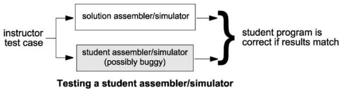
Fig. 1. Experiments run by the initial automated feedback system. The box labeled as solution assembler/simulator represents a correct program written by the instructor. The lightly shaded box indicates a program that may have a bug. The system tests a student's assembler or simulator by running it on test cases written by the instructor.
