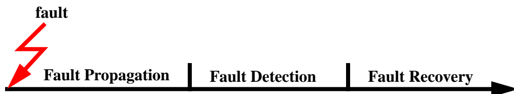
Figure 7.1 Effects of Faults During a System Crash. This figure presents a simplified version of the system-failure response stages found in [Siewiorek98].
