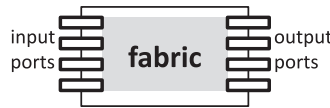
Fig. 1. Schematic switch structure. The fabric can realize a matching between the input ports and the output ports.
