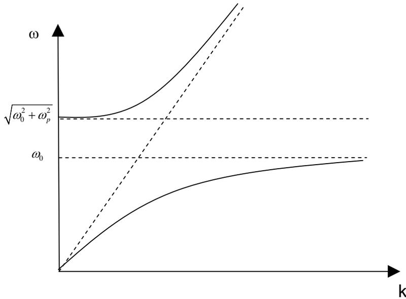
There is no density of states between  $\omega_0$  and  $\sqrt{\omega_0^2 + \omega_p^2}$ . Please explain why that is the case and what happens to an incident light with a frequency falls between these two points.
