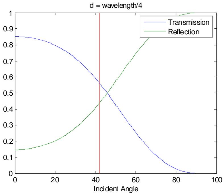
The red line represents the critical angle. We can see that by inserting the second interface, there is finite transmission through the thin slab even when the incident angle is greater than the critical angle.
