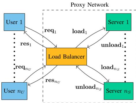
Fig. 4. The architecture of the load-balancing system.
