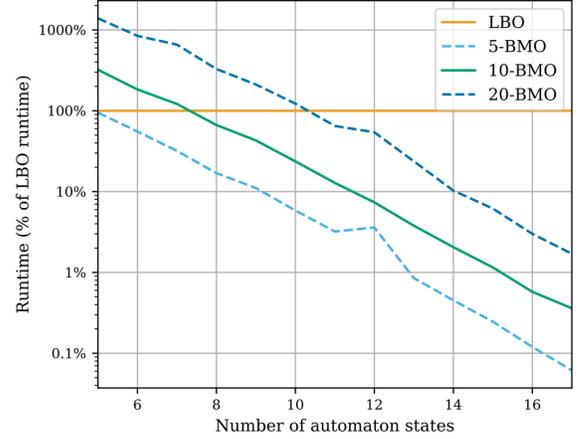
Fig. 3. The runtimes to verify different notions of opacity as a percentage of the runtime to verify LBO.
