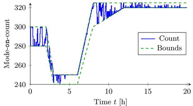
**Figure 3: Actual mode-on-count (solid blue) and imposed mode on counting bounds (dashed green) in a Simulation of Strategy 1 for an example with 1000 heterogeneous TCL's. As can be seen, the imposed bounds are satisfied throughout the simulation.**
