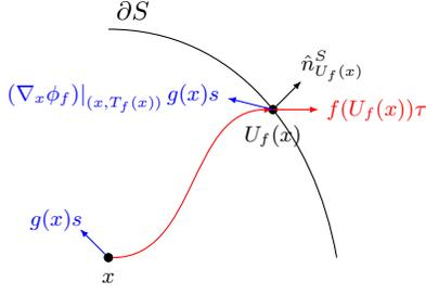
**Figure 2:** Illustration of the effect an infinitesimal movement along the vector field  $g(x)$  has on the exit time  $T_f(x)$  with respect to  $f$ . A movement  $g(x)s$  at  $x$  is propagated along the flow line of  $f$  and results in the infinitesimal movement  $\nabla_x \phi_f(x, T_f(x))g(x)s$  at  $U_f(x)$ . To compensate for this movement,  $\tau$  must be chosen so that  $f(U_f(x))\tau$  counteracts the effect in the normal direction.
