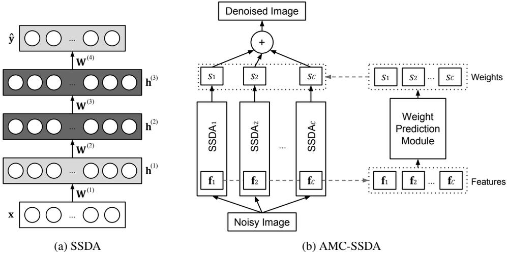
Figure 1: Illustration of the AMC-SSDA. We concatenate the activations of the first-layer hidden units of the SSDA in each column (i.e.,  $\mathbf{f}_c$  denotes the concatenated hidden unit vectors  $\mathbf{h}^{(1)}(\mathbf{x})$  and  $\mathbf{h}^{(2)}(\mathbf{x})$  of the SSDA corresponding to  $c$ -th column) as input features to the weight prediction module for determining the optimal weight for each column of the AMC-SSDA. See text for details.
