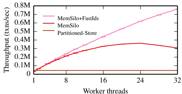
Figure 9: Performance of Partitioned-Store versus MemSilo as the number of workers processing the same size database is varied.
