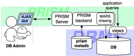
Figure 4: *PRISM* system architecture
