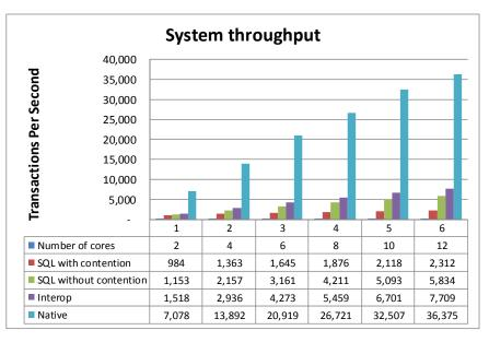
Figure 7: Experiment illustrating the scalability of the Hekaton engine. Throughput for the regular SQL Server engine is limited by latch contention.
