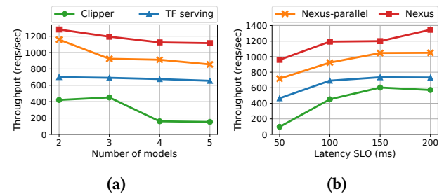
Figure 14: Impact on throughput of varying numbers of models served (a) and latency SLOs (b) under GPU multiplexing.
