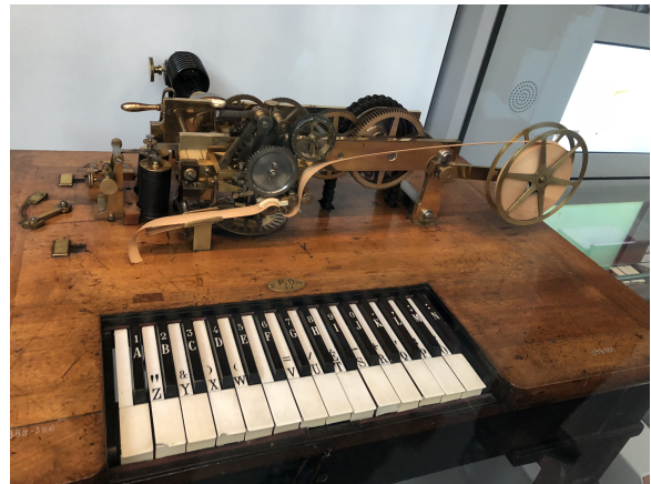
Figure 1: An 1860 Hughes' Printing Telegraph Machine.
