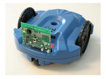
Figure 2: Parallax Scribbler with the Lancet Fluke upgrade board that provides Bluetooth, a camera, additional sensors, and LEDs.
