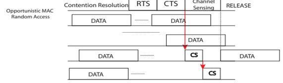
Fig. 3: O-MAC scheme: “cs” denotes channel sensing
