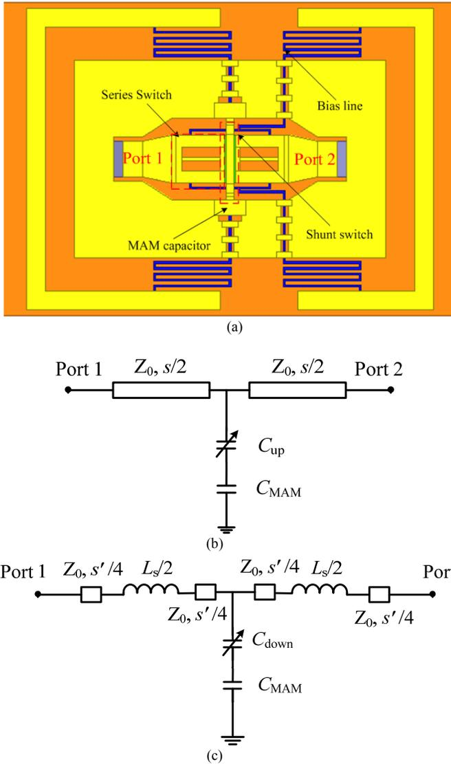
Fig. 2. The (a) structure, and (b) lumped model in the normal state and (c) in the slow-wave state for the presented DMTL phase shifter.
