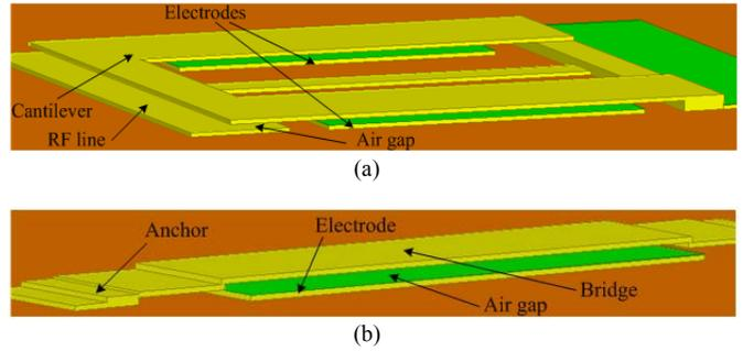
Fig. 3. The (a) structure of the series and (b) shunt switches.
