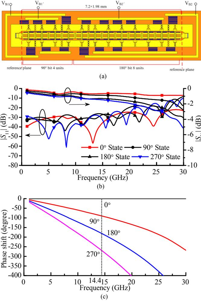
Fig. 5. (a) Layout of the 2-bit 12-section 270° DMTL phase shifter. (b)  $S$ -parameters and (c) phase shift for all states.
