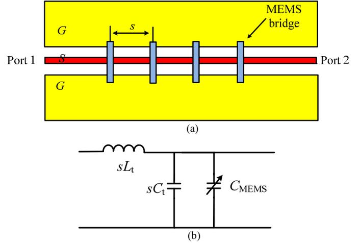
Fig. 1. (a) Structure and (b) lumped model of a conventional DMTL phase shifter. The value of  $L_t$  can be made tunable to keep the impedance matched when the capacitor is tuned.
