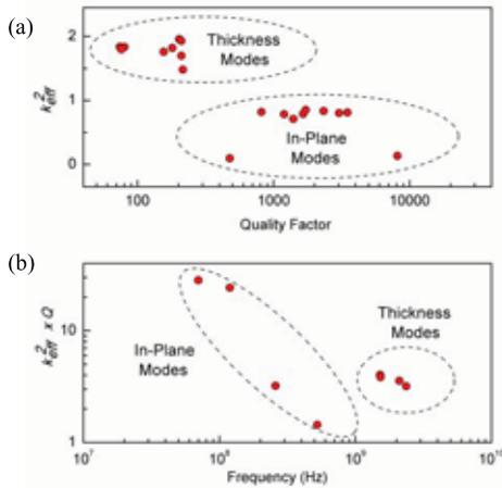
Fig. 27. Measured values of (a)  $k_{eff}^2$  as a function of and (b)  $k_{eff}^2 \times Q$  as a function of frequency. Data are taken from prior literature [17], [58]–[60].
