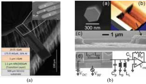
Fig. 15. (a) GaN cantilever structures (From [103]) and (b) GaN nanowires (From [107]) can be used as sensing elements utilizing the piezoresistive effect in AlGaIn/GaN 2DEG sheet. The high gauge factor of AlGaIn/GaN is due to the large modulation of the electronic properties of GaN and AlGaIn due to strain. Another major advantage of GaN piezoresistors is the ability to work at significantly elevated temperatures and still retain a high sensitivity.
