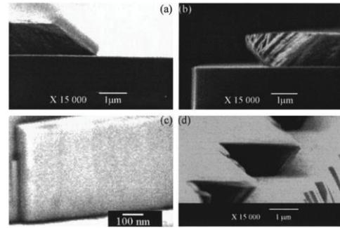
Fig. 8. Scanning electron microscope (SEM) images of crystallographic surfaces of GaN made by wet etching. (a) {1013}Plane etched by H<sub>3</sub>PO<sub>4</sub>. (b) Undercut {1012}plane etched by H<sub>3</sub>PO<sub>4</sub>. (c) Vertical {1010}plane etched by KOH in ethylene glycol. (d) Undercut {1011}plane etched by molten KOH [87].
