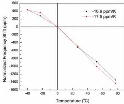
Fig. 28. The change in the frequency of two length-extensional GaN resonators as a function of temperature, showing a negative TCF with experimentally measured values of between  $-14$  ppm/K to  $-18$  ppm/K [16], [17], [89], [90].
