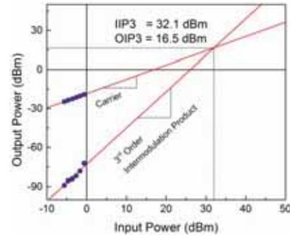
Fig. 29. Measured IIP<sub>3</sub> for a GaN mechanical resonator. The data are measured on a 2.1 GHz with a frequency separation of 50 kHz. The measured GaN bulk acoustic wave resonator shows  $Q$  of  $\sim 500$ .
