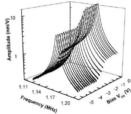
Fig. 17. Actuation efficiency versus bias voltage of an AlGaIn actuator where a 2DEG is used as bottom electrode. After [111].
