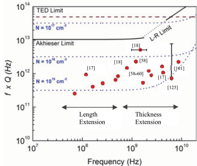
Fig. 26. Calculated values of the  $f \times Q$  limits for the dominant intrinsic dissipation mechanisms in GaN. Measured results (with error bar) from [17], [18], [58]–[60], [101], and [125].
