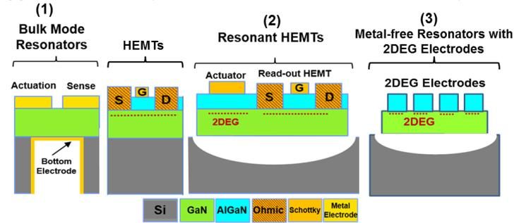
**Fig. 1.** A cross-section schematic demonstrating various types of GaN electromechanical devices discussed in this work. Functionally, these systems can act as clocks, sensors, acoustic filters/resonators, readout circuitry and communication nodes. These device types can potentially be co-fabricated on the same substrate, along with optoelectronic devices such as blue lasers and LEDs. This concept can be extended to GaN films grown on SOI substrates.
