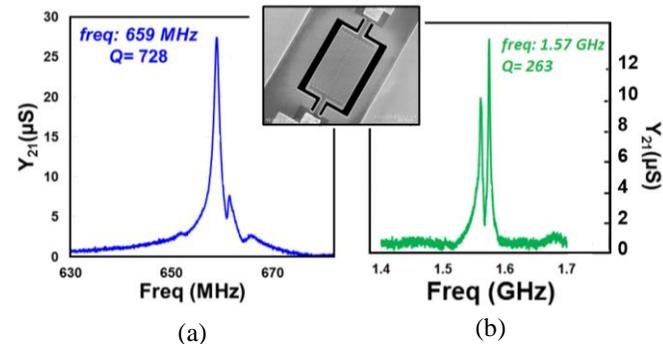
**Fig. 4.** Resonators with 2DEG electrodes
