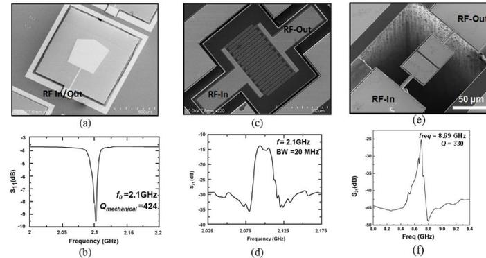
**Fig. 2.** Bulk mode resonators
