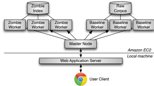
Figure 2: The IDE’s basic runtime architecture.
