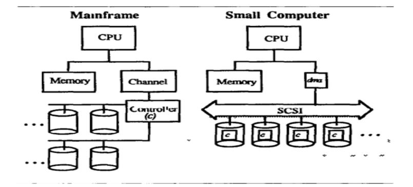
•Same SCSI interface chip embedded as a controller in every disk can be used as the DMA device at the other end of the SCSI bus.
