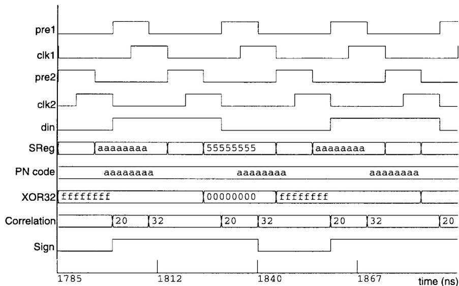
Fig. 21. Functional simulation of correlator in verilog.
