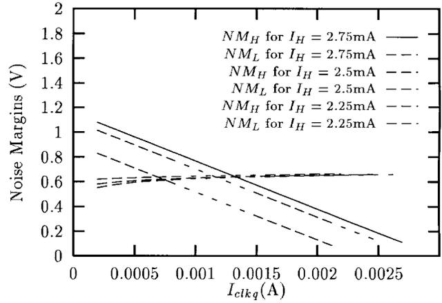
Fig. 6. Noise margins versus  $I_{clkq}$  for different  $I_{clkh}$ .
