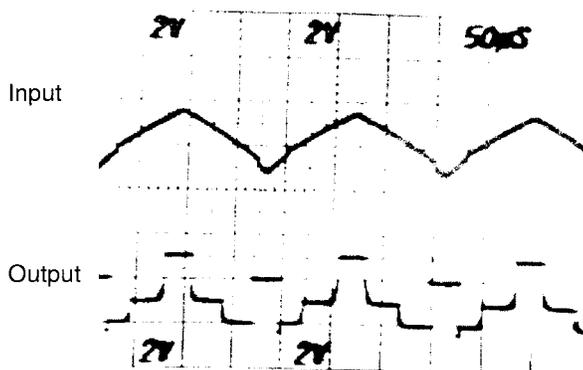
Fig. 31. Experimental result of MVL programmable gate.
