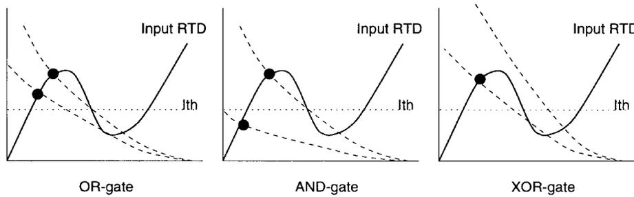
Fig. 13. Load lines for RITD-based logic function circuit.
