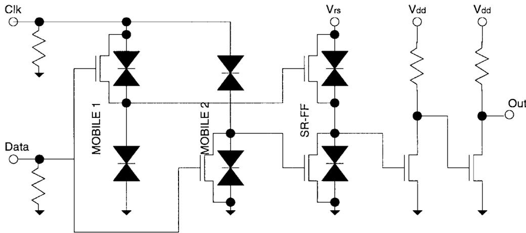
Fig. 16. Circuit configuration of a MOBILE-based D-FF.
