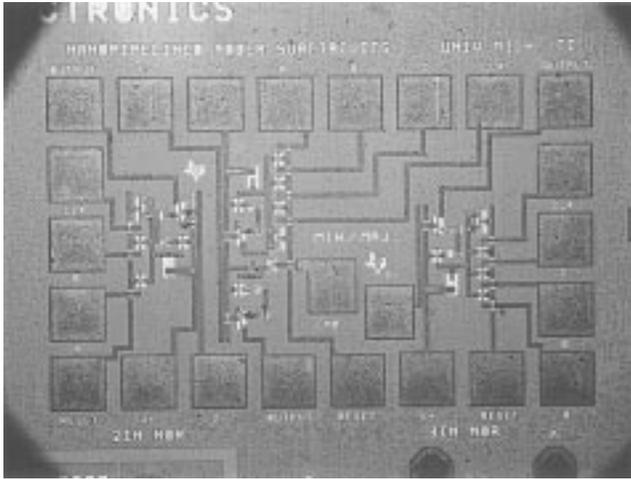
Fig. 10. Photomicrograph of RTD + MODFET logic circuits chip.
