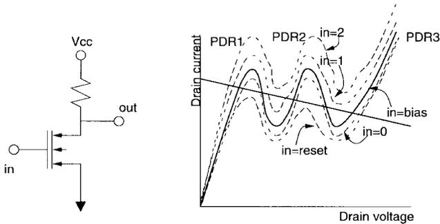
Fig. 26. MJ-STT tristable circuit and load lines.
