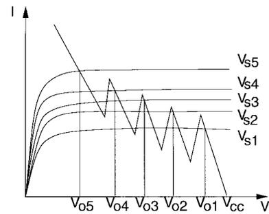
Fig. 33. Load lines for the multivalued counter.
