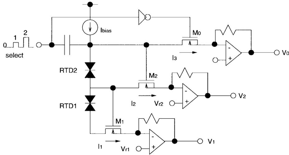
Fig. 25. RTD-based multiple-valued decoder circuit.
