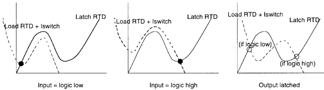
Fig. 12. Load lines for RITD-based latch circuit.
