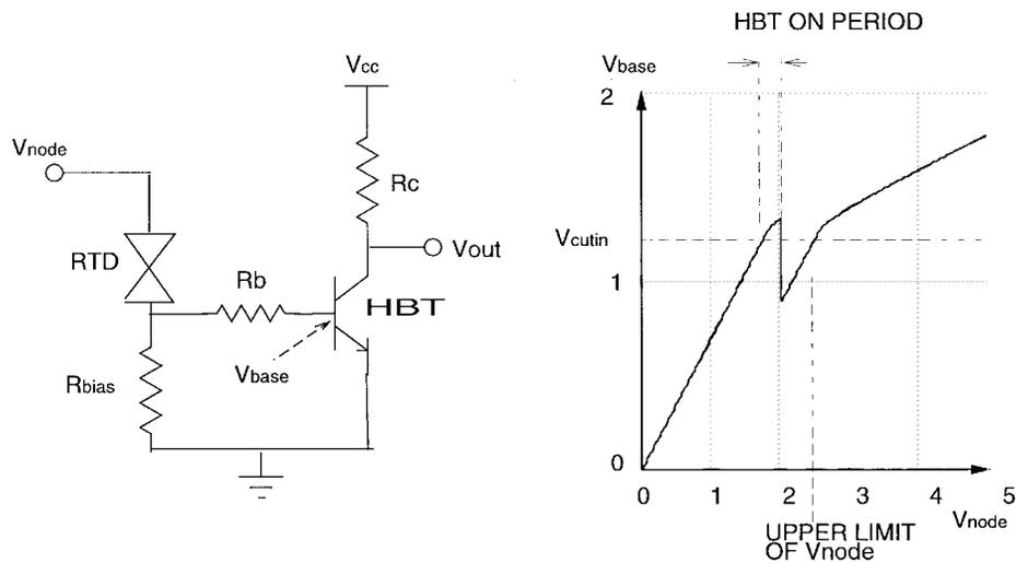
Fig. 27. RTD selector circuit and operating principle.
