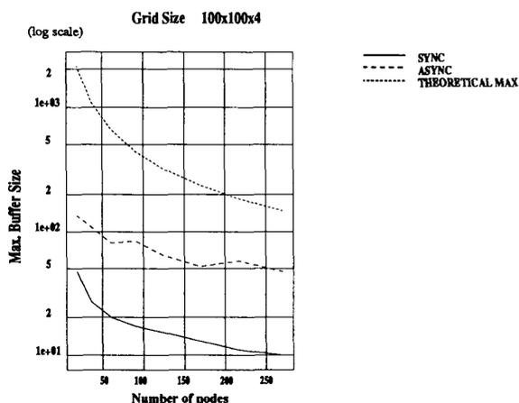
Fig. 17. Determination of maximum buffer store size needed.
