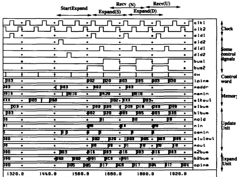
Fig. 13. Simulation trace for the HAM processor.
