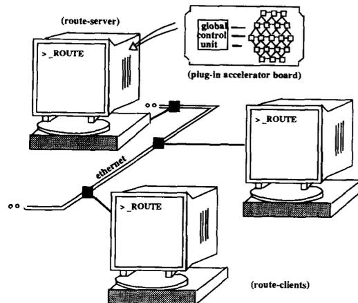
Fig. 3. Overview of the HAM routing system.
