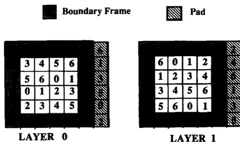
Fig. 6. Padding scheme for a 2-layer  $4 \times 4$  grid.
