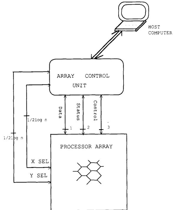
Fig. 7. Overview of the hexagonal array machine.
