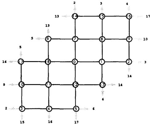
Fig. 12. Four-dimensional hexagonal array with diagonals links removed.
