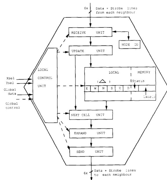
Fig. 8. Block diagram of a single processing element.
