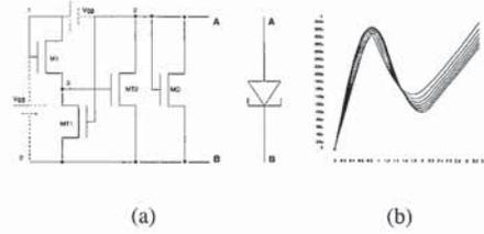
Figure 2: (a) Four transistor RTD emulator showing two possible positions of  $V_{gg}$ . (b) I-V characteristics of MOSFET NDR circuit.
