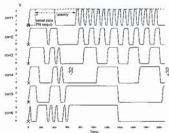
Figure 7: Simulation result showing correlation value changing from  $-32$  to  $+32$  in response to serial data input change.
