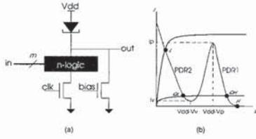
Figure 1: (a) Bistable-mode QMOS logic gate (b) Load lines for bistable QMOS gate operating point
